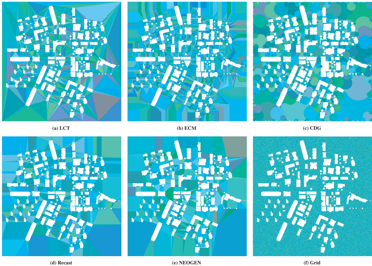
Fig. 17. Navigation meshes computed for the City environment. Regions are shown in different colors.
